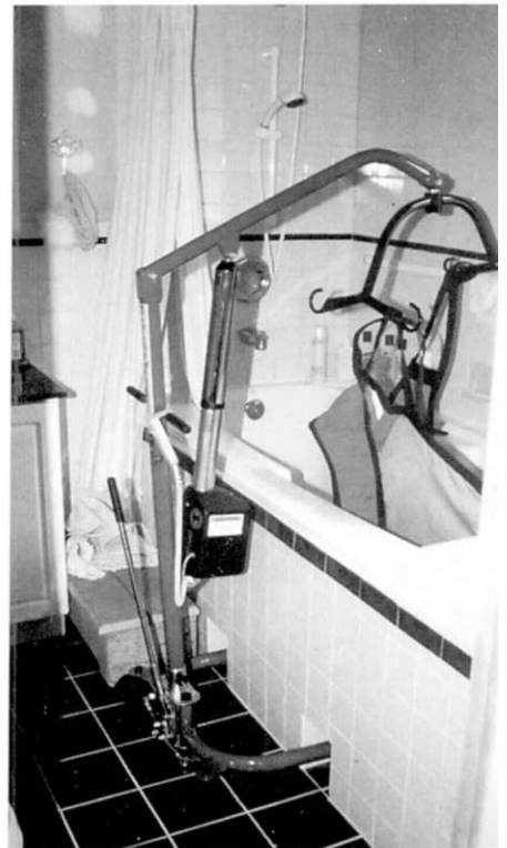
Space underneath tub for legs of lift keeps the lift balanced.
