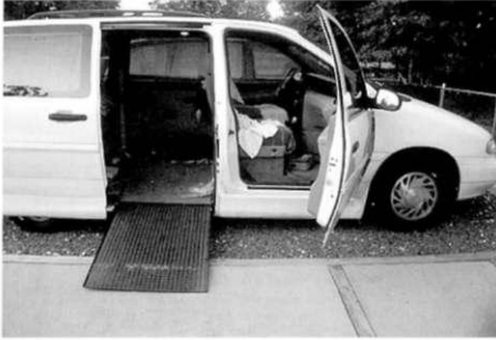
A flat, level sidewalk provides an accessible receiving surface for a lift.
