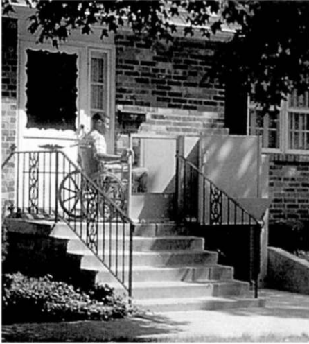
Outdoor lifts are particularly good for homes with small lots and insufficient room for a ramp. They can also be dismantled and moved to a new location.
